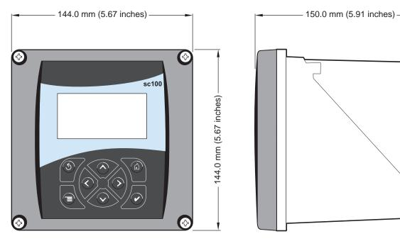
Figure 3-3 Controller Mounting Dimensions
